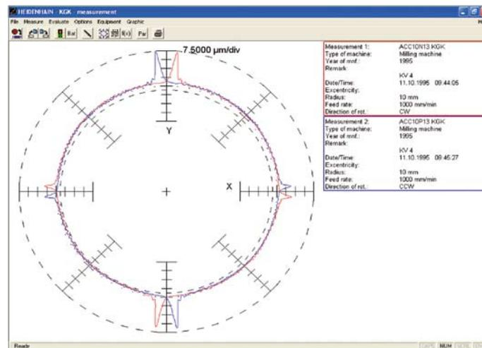
Standardized representation of a circular interpolation test with a KGM: The reversal peaks at the quadrant transitions are visible, as is the difference between clockwise and counterclockwise traverse
