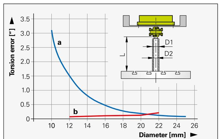
Torsion error of the 100 mm long coupling of an ROD 880 through a
