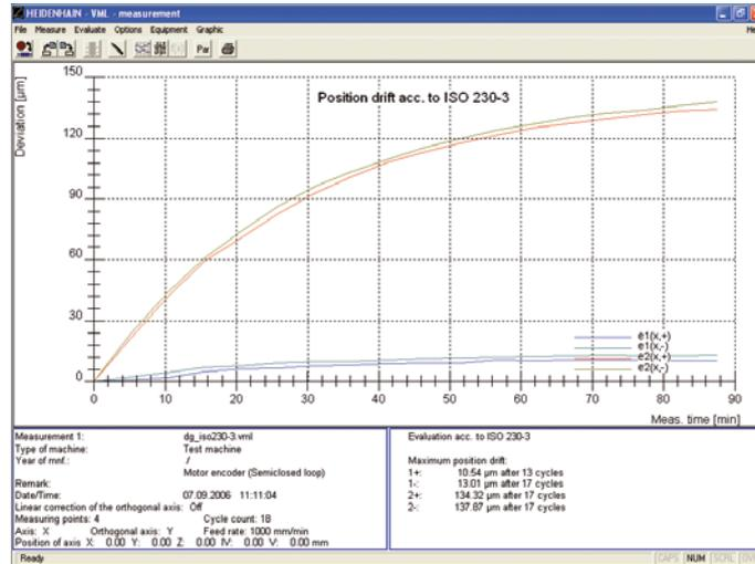
Determining the **thermal behavior** of a linear axis as per ISO 230-3 measurement with the VM 182 and feedback via the rotary encoder in the motor ("Semi-Closed Loop") ...
