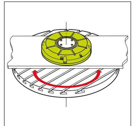
The position accuracy and repeatability of rotary axes, rotary tables and tilting tables can also be determined. A very precise angle encoder serves as comparator system.
